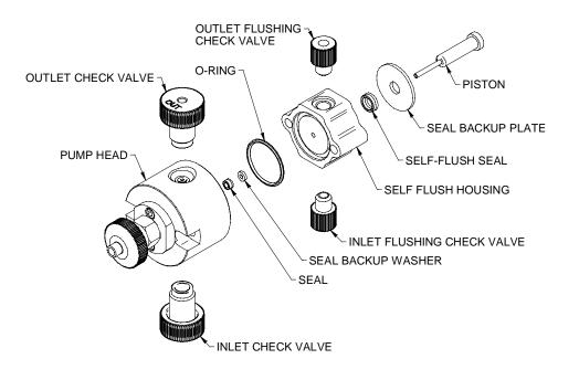
Figure 5-3. Bioclean (PEEKTM) Self-Flushing Pump Head Assembly
